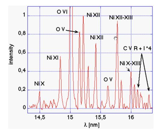
Experimental and simulated M-shell nickel spectra in the 14.4–18.0 nm region from magnetic fusion devices Mattioli et al. J. Phys. B: At. Mol. Opt. Phys. 37 (2004) 13–40
