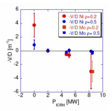
Fig.4 Ni peaking factors at  $\rho=0.2$  and  $\rho=0.5$  versus ICRF powers for the 6 discharges, Mo peaking factors for shot #68381. New proposals for 2008: - look for a power threshold for the pinch inversion - include W - compare data
