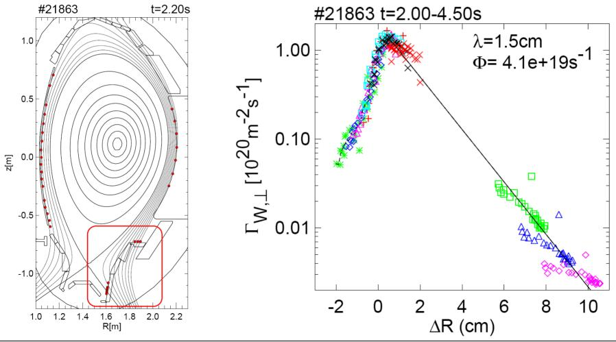
W-erosion decreases with increasing level of gas puff (recycling) leading to lower temperatures in divertor
