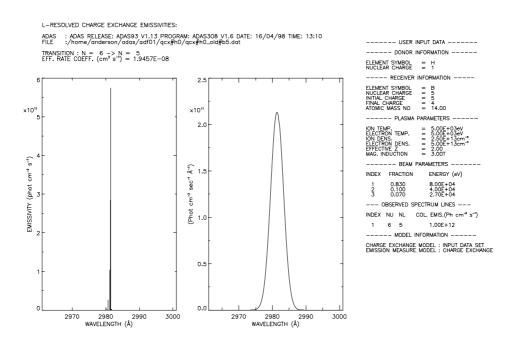
The analysis of charge exchange emission by the code is shown in figure 4.8a and table 4.8a. Emission following electron capture by  $B^{+5}$  from neutral deuterium beam atoms in their ground state is illustrated. A single observed line-of sight emissivity in the transition BV (n = 6 ---> n = 5) is analysed. Figure 4.8a shows the theoretical breakdown of emission in the above line into multiplets and the expected Doppler broadened profile of the feature
