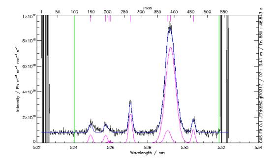
Figure 1: Example of composite CVI spectrum observed for JET shot 70312. The CVI temperatures of the active (ACX) and passive (PCX) components are 2811eV and 823eV respectively.
