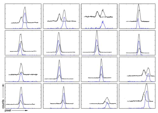
Fig 2.40: The HeI (587.6 nm /  $2^{1}$ P- $3^{3}$ D) spectra measured in the pulse JPN 49555 for 16 viewing lines. In each graph the spectrum measured during a beam on phase (t = 61.3 s), the background spectrum (linear interpolation of the spectra from t = 61.2 and 61.4 s), and the difference between the two (blue) are plotted.
