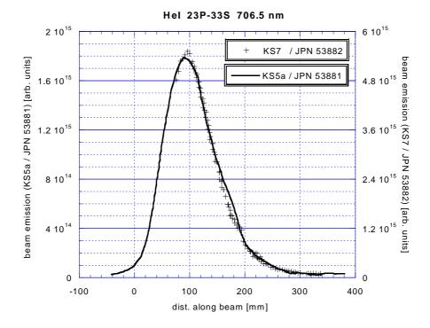
Fig. 2.46: Comparison of HeI 2<sup>3</sup>P-3<sup>3</sup>S (706.5 nm) beam emission profiles taken from comparable plasma pulses with different He beam energy. KS5a observed a 135 keV doped He beam and KS7 a 73 keV pure He beam.
