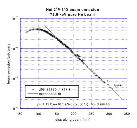
Fig. 2.50: Triplet HeI beam emission  $2^{3}P-3^{3}D$  at 587.6 nm for injection of a pure He beam (JPN 53879), plotted on a logarithmic scale. The solid line is an exponential fit to the decay inside the plasma.
