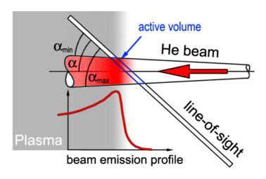
Fig 3.6: Sketch of the influence of the finite beam divergence on the net Doppler-shift.
