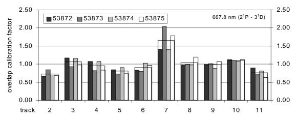
Fig. 2.19: Overlap-calibration-factors for four successive pulses with the spectrometer set to 667.8 nm.
