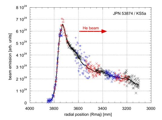
Fig. 2.22: Emission profile for the HeI singlet line 667.8 nm  $(2^{1}P-3^{1}D)$ . The symbols are data (spaced 2 mm) resulting from the fit of single frames (50 ms exposure time). The solid line gives an average over 10 data points, corresponding a distance of 20 mm.
