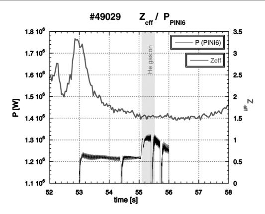
Fig. 2.35: Time trace of the mean  $Z_{eff}$ , together with the injected beam power from the He doped PINI. During and after the He injection no increase in  $Z_{eff}$  can be seen.
