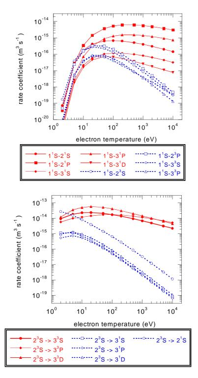
Fig. 1.1: Electron temperature dependence of rate coefficients for electron impact excitation out of the He ground state (1<sup>1</sup>S) into several excited levels.
