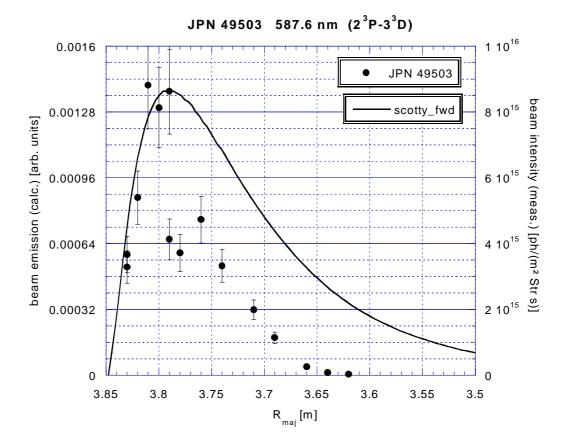
Fig. 2.38: Beam emission profile of the 587.6 nm He I line  $(2^{3}P-3^{3}D)$  measured during the pulse JPN 49503. The intensities of the two tracks at the radial position  $R_{maj} = 3.81$  m and 3.82 m are too low, indicating an incorrect calibration.
