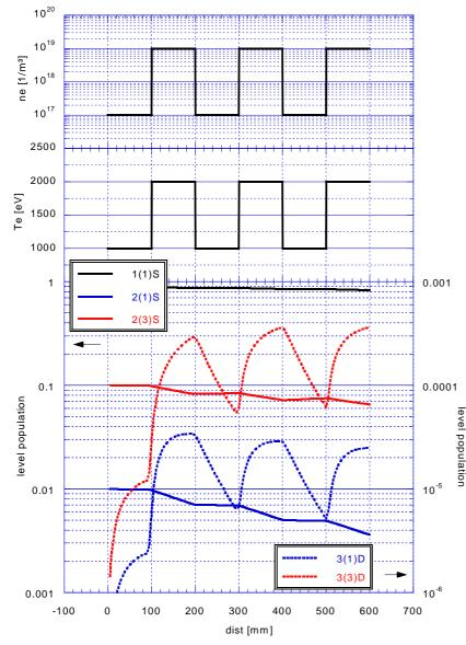
Fig. 2.56:  $n_e$ - and  $T_e$ -Testprofiles (periodic square profile) and the modelled population of some HeI levels. The resulting emission profiles show the expected spatial correlation, indicating correct calculation of the output distance.
