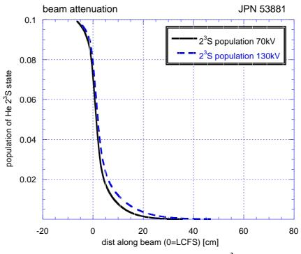
Fig. 2.21: Modelled beam attenuation of the 2<sup>3</sup>S level for two different beam energies.
