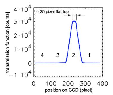
Fig. 2.36: The transmission-function of one slit (second of the first row). The numbers 1 ... 4 indicate the position of all four transmission function of the first row of the slit-array.
