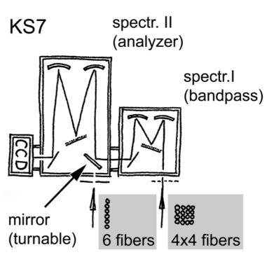
Fig. 2.7: Schematic view of the KS7 spectrometer with two spectrometers in series ("standard mode" of operation).
