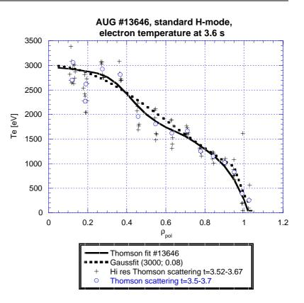
Fig. 2.25: Electron temperature profile for the standard H-mode discharge #13646 at t = 3.6 s. Symbols are straight data from Thomson scattering (standard and high resolution), the fit is from the standard Thomson scattering. Data points and Thomson fit show a centrally peaked profile. However, also a Gauß fit is consistent with the data due to its large scatter.
