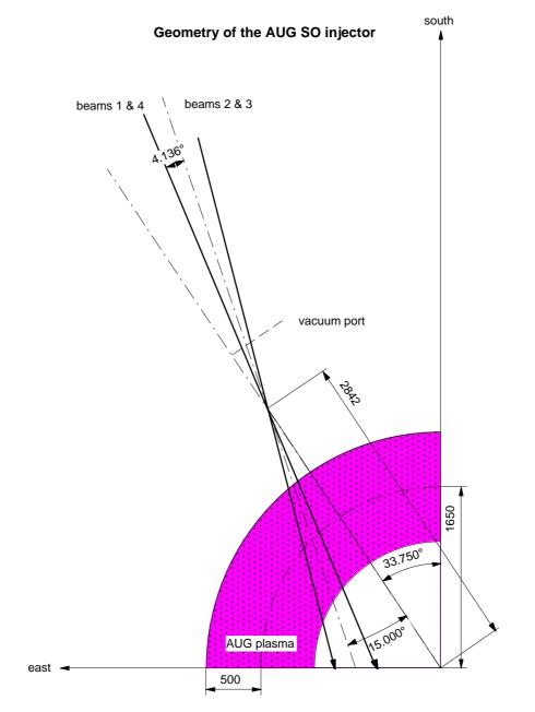
Fig. 3.10: Geometry of the AUG 60 kV injector. He beam emission measurements were performed with beam 3.
