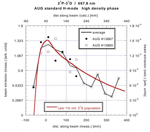
Fig. 2.29: Beam emission measurements (AUG #13667, #13880, and average) and modelling of the HeI line  $(2^{1}P-3^{1}D)$ . The two abscissas (meas. and calc.) were shifted against each other by 40 mm.
