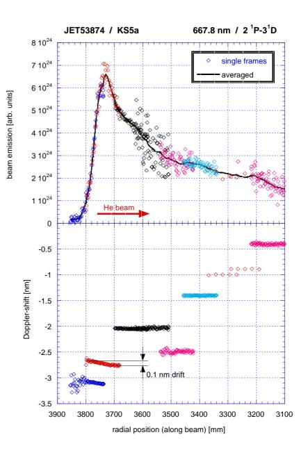
Fig 3.7: Intensity and Doppler-shift of the HeI  $(2^{1}P-3^{1}D)$  beam emission measured during a sweep experiment. At the location with high emission gradient a changing Doppler-shift is noticeable.
