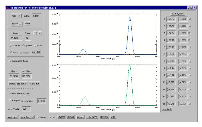
Fig. 3.3: Screen shot of the main widget of the IDL-program he\_wid
