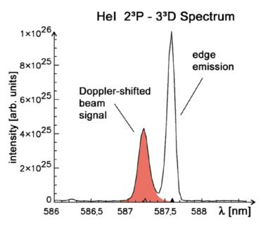
Fig 3.1: HeI beam emission spectrum of the 2<sup>3</sup>P-3<sup>3</sup>D transition (587.6 nm).
