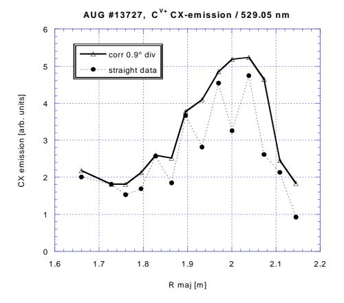
Fig. 3.11: The zigzag of the data retrieved with the "cer-wid" evaluation software disappears if the intensities are corrected by the beam intensity at the crossover between beam and viewing line. Assumed beam divergence:  $0.9^{\circ}$ .
