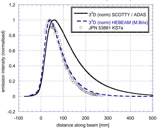
Hel beam emission 2<sup>3</sup>P-3<sup>3</sup>D (587.6 nm)
