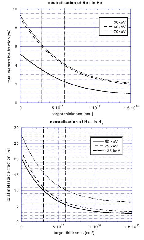
Fig. 2.52+2.53: Total metastable fraction  $(2^{1}S + 2^{3}S)$  of He beam obtained by neutralisation of He<sup>+</sup> in a gas target for different beam energies. The probable target thickness range of the JET neutraliser is indicated by dotted lines.
