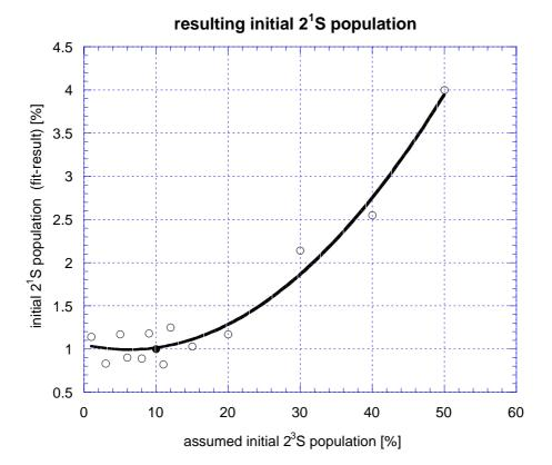
Fig 4.8: Initial metastable singlet population  $(2^{1}S)$ , derived by the yttocs code, for synthetic data generated with initial metastable populations of 1% singlet  $(2^{1}S)$  and 10% triplet  $(2^{3}S)$  states (solid black dot). The open points represent the derived initial singlet population for a given initial triplet population. For up to 20%  $2^{3}S$  population not much difference of the  $2^{1}S$  population is found.
