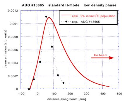
Fig. 2.27: Beam emission measurement and modelling of the HeI transition  $2^{3}P-3^{3}D$  (587.6 nm) for the AUG discharge #13665. The obvious discrepancy in the curve width is discussed in chapter 2.6.3.
