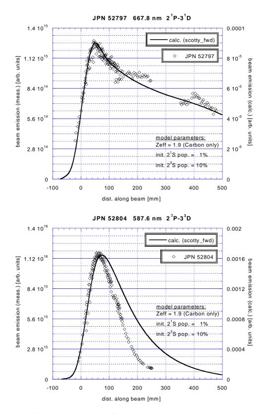
Fig. 2.41: He beam emission profiles from a doped 70.3 keV He beam observed with KS7, compared with model calculations (scotty\_fwd). Upper graph: JPN52797, HeI singlet line (2<sup>1</sup>P-3<sup>1</sup>D) at 667.8 nm Lower graph: JPN52804, HeI triplet line (2<sup>3</sup>P-3<sup>3</sup>D) at 587.6 nm
