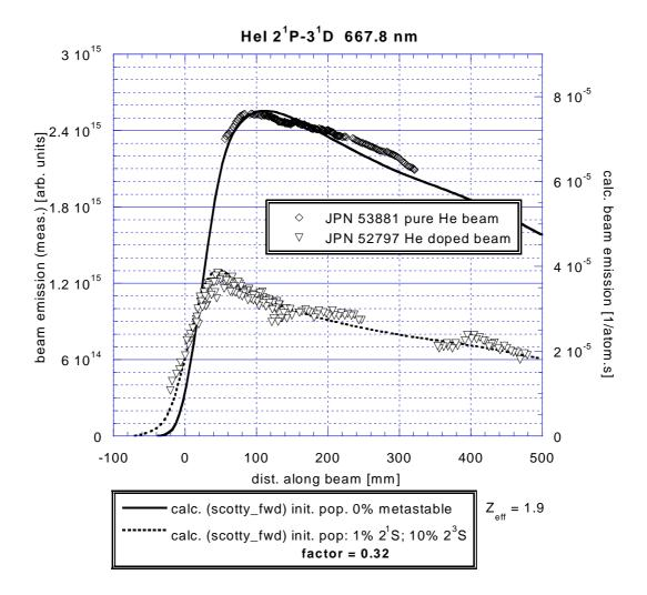
Fig. 2.51: He beam emission of the  $2^{1}P-3^{1}D$  transition at 667.8 nm measured with pure and a doped helium beams. The modelled beam emission was calculated for an initial metastable  $2^{1}S$  population of zero in the case of the pure beam and of 1 % in the case of the doped beam.
