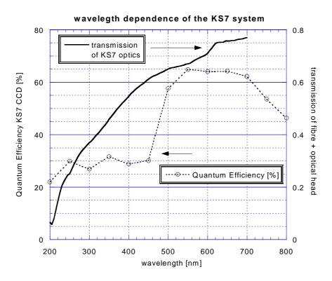
Fig. 2.33: Measured quantum efficiency of the KS7 CCD sensor and calculated transmission of the optical system.
