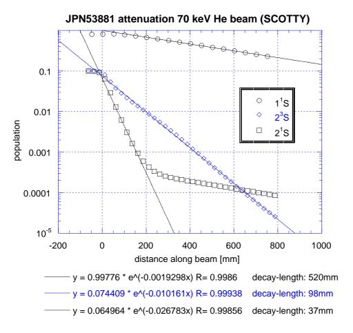
Fig 4.7: He beam attenuation of initially populated levels, modelled for the JET discharge 53881.
