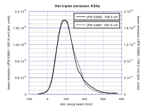
Fig. 2.45: Comparison of the beam emission profile for the  $2^{3}P - 3^{3}D$  transition at 587.6 nm (JPN 53881) with the one for the  $2^{3}P - 3^{3}S$  transition at 706.6 nm (JPN 53882).
