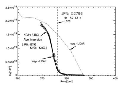
Fig. 2.12: Density profiles for a series of identical L-mode sweep pulses derived by the Abel-inversion of edge-interferometer data during sweeping
