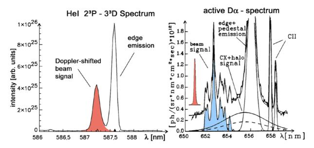
Fig. 2.3: Comparison of the  $2^{3}P-3^{3}D$  (587.6 nm) HeI beam emission spectrum (left graph) with the  $D_{\alpha}$ -spectrum (right graph). The shaded peaks (He red and D blue) results from the respective excited beam particles.
