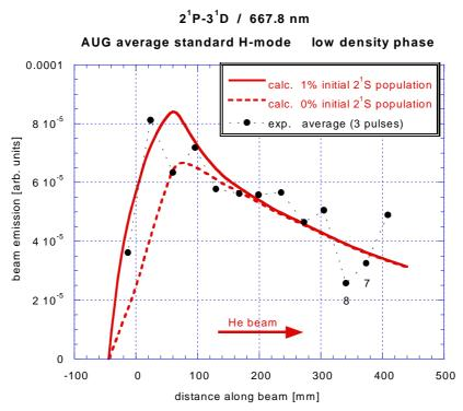
Fig. 2.26: He beam emission measurements (average over AUG #13646, #13667, #13880) and modelling of the HeI transition  $2^{1}P-3^{1}D$  (667.8 nm). The measurements can be reproduced by the model calculations if an initial population of the  $2^{1}S$  state of 1% is assumed.
