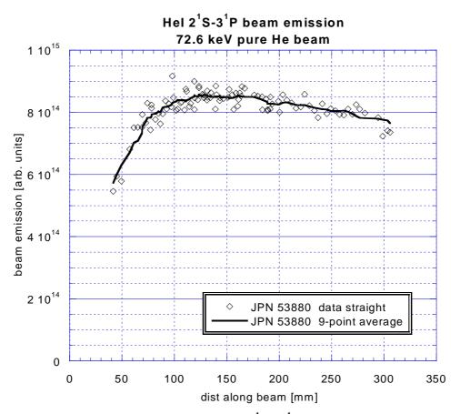
Fig. 2.47: HeI emission profile from the  $2^{1}S - 3^{1}P$  singlet line at 501.5 nm.
