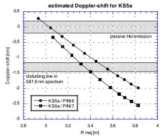
Fig. 2.11: Estimated Dopplershifts for the KS5a viewing lines for the 587.6 nm (2<sup>3</sup>P-3<sup>3</sup>D) beam emission coming from a 140keV He beam (PINI 6 and PINI 7).
