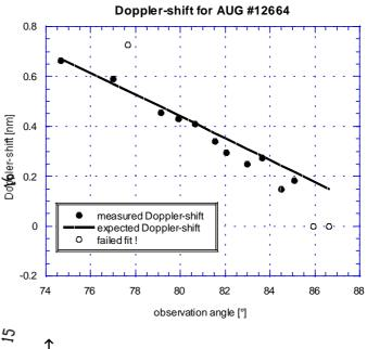
Fig. 2.5: Expected (solid line) and measured (dots) Doppler-shift of 667.8 nm (2<sup>1</sup>P-3<sup>1</sup>D) HeI beam emission observed during AUG pulse #12644. The open dots are used for tracks, where the fit procedure failed.
