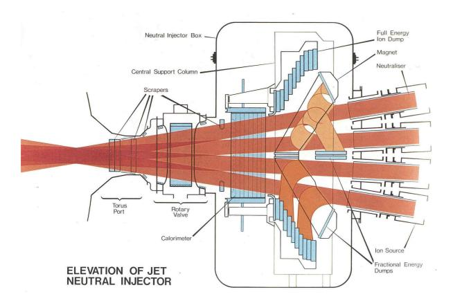
Fig. 2.1: Side view onto the JET neutral beam injector.
