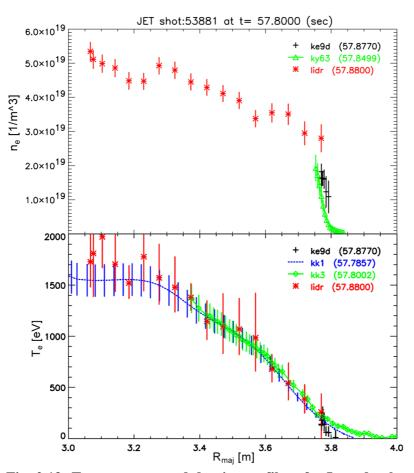
Fig. 2.13: Temperature- and density profiles of a L-mode plasma used for the sweep experiments, as measured with the standard diagnostics.
