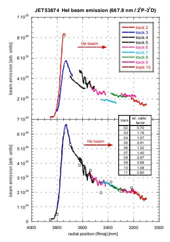
Fig. 2.18: Upper graph: Data shown in Fig. 2.17 mapped to respective major radius at t= 58 s. Lower graph: Same data after "overlap"-calibration.
