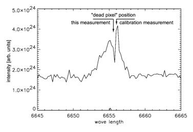
Fig. 3.8: Example of a spectrum with a dead pixel within the Doppler-shifted peak.
