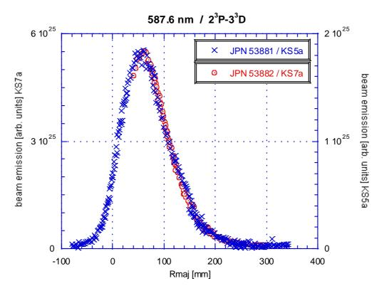
Fig. 2.20: Profile of the emission of a HeI triplet line measured with the spectrometer KS7 looking at a 75 kV beam and with KS5a looking at a 135 kV beam, for two repetitive pulses. The profile measured with KS7 was shifted radially by -20 mm against the other profile.
