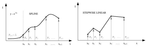
Fig 4.2: Examples for the parametrisation of the profiles.  $P_i$  are the parameters changed by the fitting-procedure. In both examples they are restricted to positive values. The  $x_i$  are the fixed spatial positions of the knot points.
