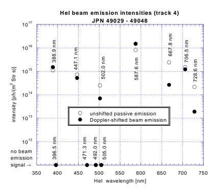
Fig. 2.31: Intensity of the Doppler-shifted HeI beam emission peaks (solid dots) and the corresponding unshifted passive emission (open symbols). Wavelengths where no beam emission signal could be identified are indicated on the abscissa.
