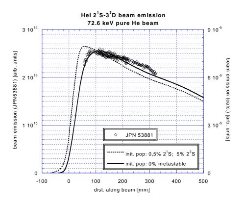
Fig. 2.48: Comparison of the measured  $2^{1}P-3^{1}D$  transition (667.8 nm) with model calculations. The two lines are calculations assuming either 0 % (solid line) or 0.5 % (dashed line) initial  $2^{1}S$  population of the He beam.
