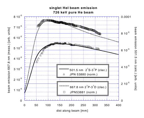
Fig. 2.49: Comparison of the  $2^{1}$ S -  $3^{1}$ P singlet line profile at 501.5 nm with the profile from the  $2^{1}$ P- $3^{1}$ D transition (667.8 nm). The plasma discharges are comparable, and for both discharges a pure He beam was used.
