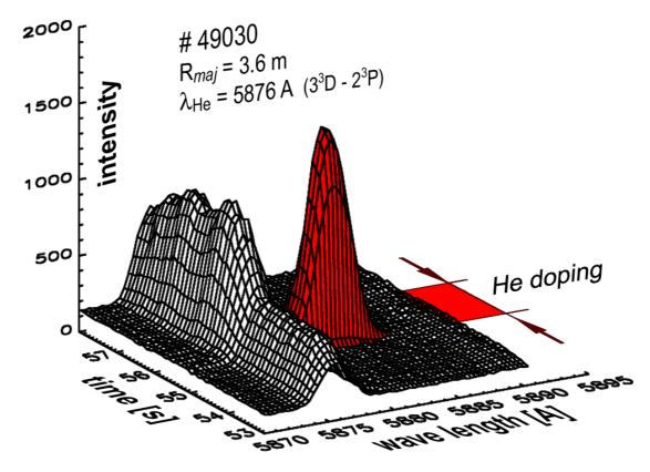
Fig. 2.34: Time development of a HeI spectrum recorded for one viewing-line. The appearance of the Doppler-shifted beam emission peak (red) indicates the time of He doping. At the same time the unshifted peak from the passive edge emission increases.
